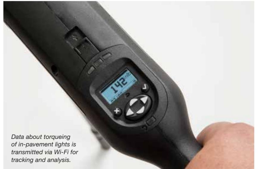
Data about torquing of in-pavement lights is transmitted via Wi-Fi for tracking and analysis.
